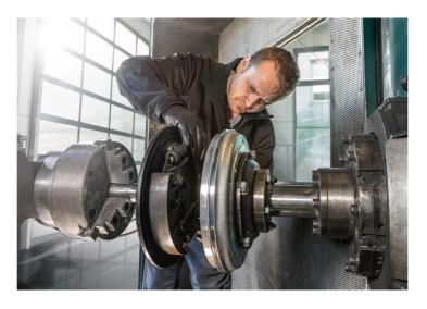
compromise solutions was good enough for a 356 A. The new edition now offers 356 A owners a much better solution: a new 356 A brake drum re-manufactured according to the original plans with the original look. And just like the original 356 A brake drum, the new edition is also 'Made in Austria'.
