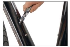
Please keep in mind that the material is particularly sensitive to pressure when using clamps [e.g. seat and derailleur clamp]. Always use a torque wrench and observe the specified tightening torques [see "Recommended tightening torques", p. 78].
