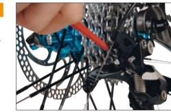
Location of the limit stop screws to the inner and outer stop position may differ with the shifter. For this reason, please be absolutely sure to observe additional instructions of the shifter manufacturer.
