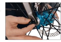
For this, open the guick release again and tighten the nut more in a clockwise direction. Close the quick release and again check that it is securely positioned.
