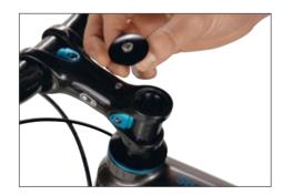
Install the stem by placing it on the fork shaft. Place the spacer rings you removed over the stem onto the fork shaft.
