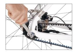
Follow the steps in reverse order to mount the tyre. Use a torque wrench to mount the wheel.
