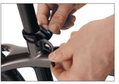
To adjust the seat height, open the quick release of the seat post clamp.
