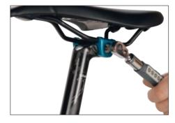
Now push the seat into the desired position to the front or back. Pay attention to the marks on the seat rails and do not move the seat past them.
