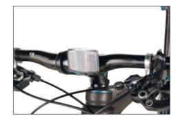
Once the clamp is securely positioned on your handlebar, push the white reflector RR-180-SL onto the holder
