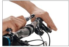
reach, make sure there is adequate space for applying the brake pads to the brake discs without the brake lever coming into contact with the handlebars.
