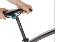
You can set the seat incline and seat position in addition to the seat height. By adjusting the seat position, you change the distance to the handlebars and your pedalling position above the pedal crank. The seat incline should be as levelled as possible so that the cyclist is able to pedal comfortably without slipping off the seat.
