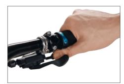
Normally, you operate the large lever with your thumb. The smaller lever in front of the handlebars is operated with your index finger or thumb [Shimano Syfront forke with 2-way release].
