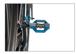
The pedals are labelled "R" for the right pedal and "L" for the left pedal. Consult the table "Recommended tightening torques" on p. 78 or the documentation of your pedal manufacturer for the required tightening torques.
