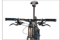
Hydraulic disc brakes are very effective and it is easy to overestimate how much pressure is needed to activate them. For this reason, you should test their effectiveness on a level, non-slip track that is removed from road traffic. Please read the chapter "Brakes" on p. 32 carefully.
