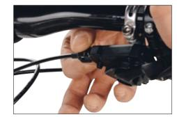
When making the first fine adjustments, try turning the adjusting screw counter-clockwise to compensate for the stretching. Make gradual adjustments with the adjusting screw. Check the adjustment by shifting one gear up and then back down. If this is successful, shift through all gears on the cassette in both directions.
