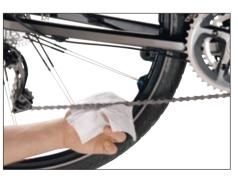
Despite regular care, the chain is still subject to wear and tear. The lifecycle of chains normally corresponds to approximately 800 - 2500 km or 40 - 125 hours of use. Replacing your chain regularly can extend the lifecycle of your chain rings and your cassette.
