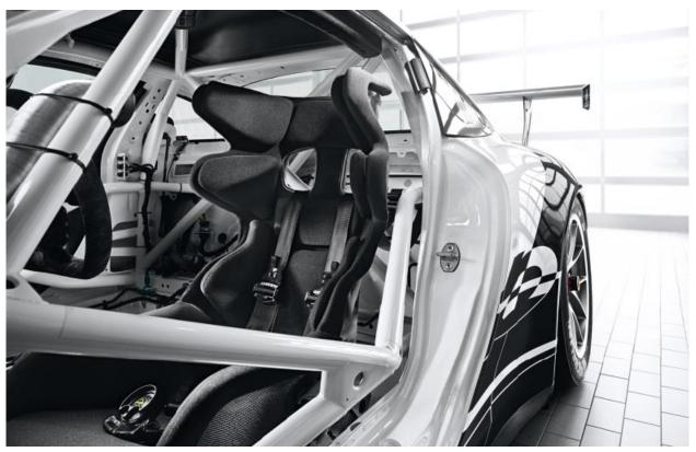
Within the realm of possibility: In the event of a roll-over or collision, a newly developed roll cage protects the occupants
