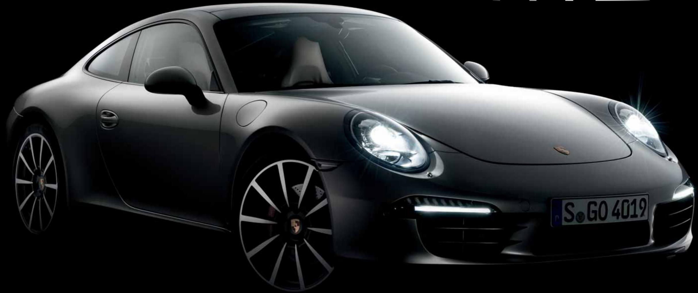
WHEELBASE: 10 CM (3.93 INCHES) LARGER; CHASSIS: 56 MM (2.2 INCHES) LONGER; OVERHANG FRONT AND REAR: SHORTENED; ROOF LINE: 7 MM FLATTER; TRACK: WIDER. **THE NEW 911.**
