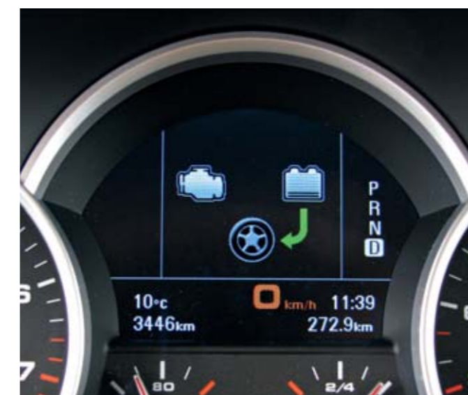
Electric drive: The green arrow shows that the electric motor is currently powering the wheels
