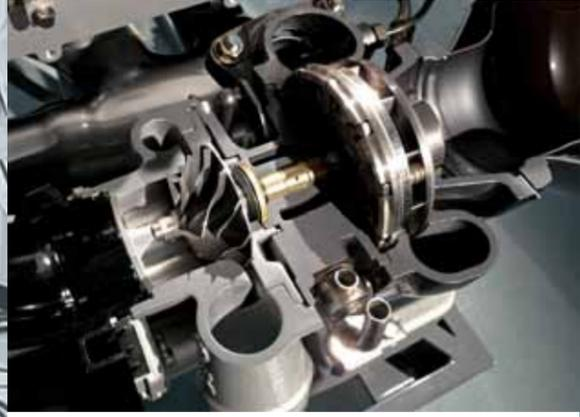
Turbocharging with dual chargers with variable turbine geometry in a symmetrical arrangement
