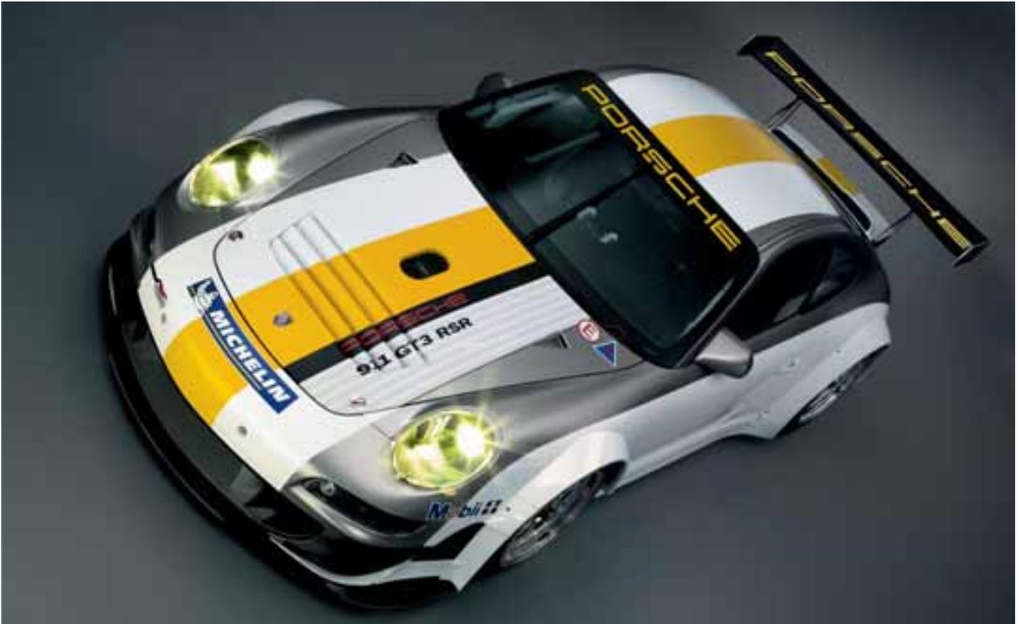
engine management system that adapts even better to the corresponding fuel grades, as well as from a newly designed exhaust system and a reworked air-intake housing. Modifications to the front area are noticeable right away. A new front lip increases downforce on the front axle, and the front wheels are wider with the rims now measuring 12 instead of 11 inches, which ensures better grip and a reduced tendency to understeer. The rear-wing placement and the
