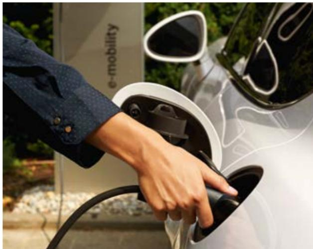
Plug-in: Charging at an electrical outlet takes two and a half to four hours
