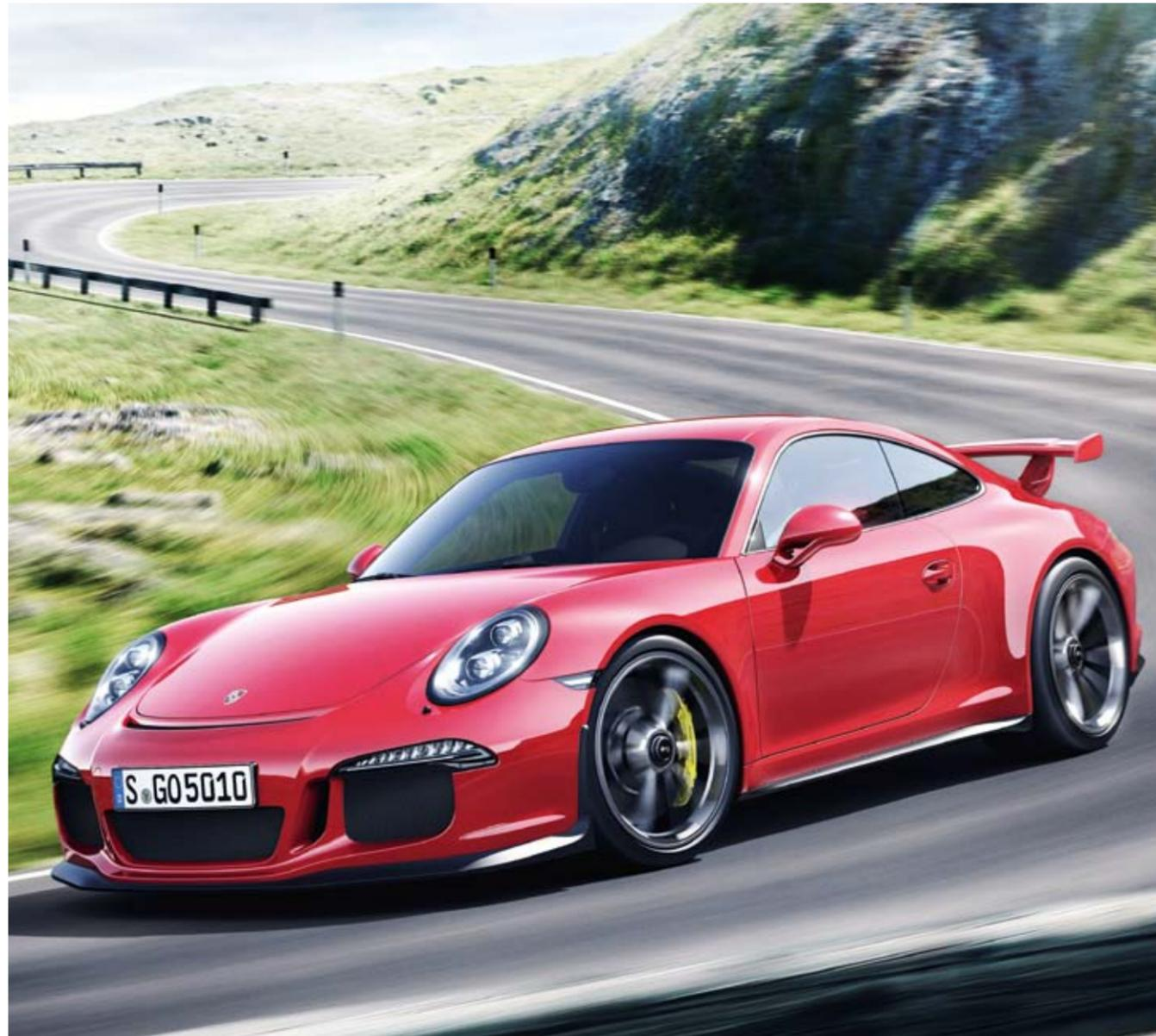
*With its wheelbase lengthened by 3.9 inches, the new 911 GT3 drives as if on rails. The wider front track gives it even greater agility and stability in curves.*
