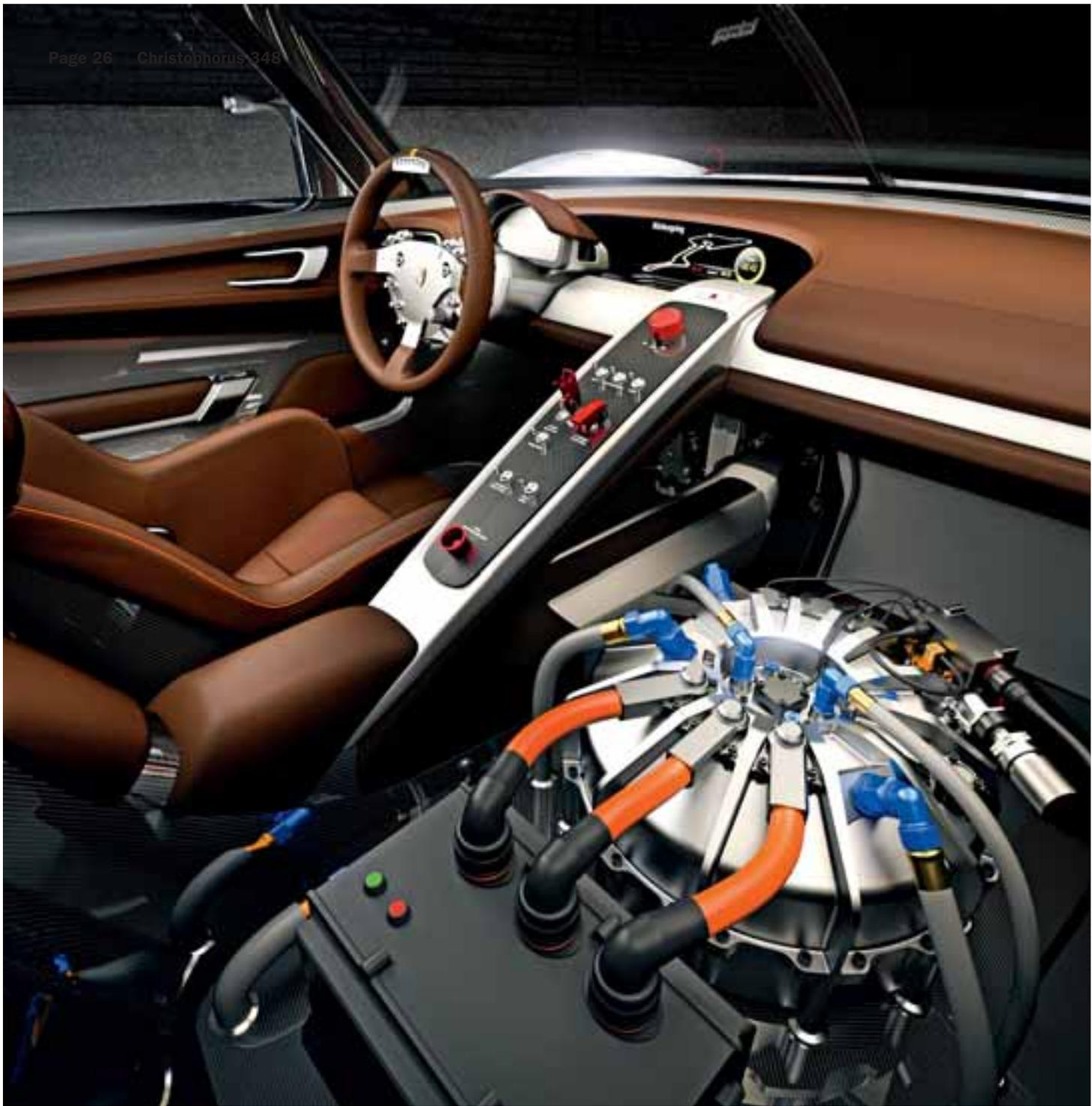
During braking maneuvers, the flywheel absorbs energy, which then provides additional acceleration power via the electric motors on the front axle
