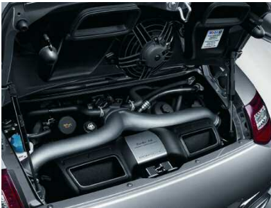
Inside view: The 3.8 litre engine of the seventh Turbo generation produces 500 HP (368 kW)
