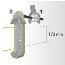
Fig. 6: Drilling dimensions
