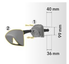
Fig. 8: Drilling dimensions
