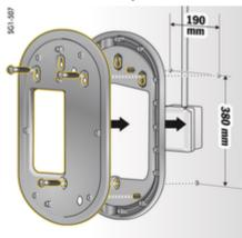
Fig. 12: Drilling dimensions
