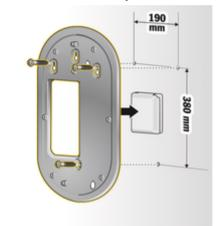
Fig. 10: Drilling dimensions
