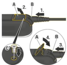
Fig. 16: Connecting cable and securing plug
