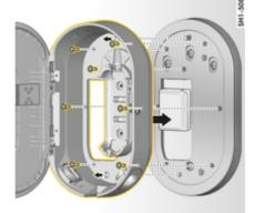
Fig. 13: Screwing charging dock to assembly plate
