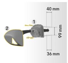
Fig. 8: Drilling dimensions
