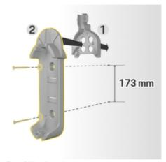
Fig. 6: Drilling dimensions
