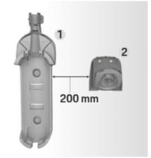
Fig. 7: Distance between wall mount and connector fastener
