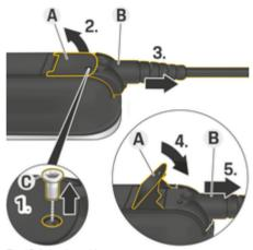
Fig. 15: Releasing cable
