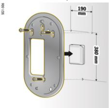
Fig. 10: Drilling dimensions
