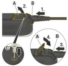
Fig. 16: Connecting cable and securing plug
