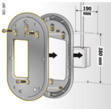
Fig. 12: Drilling dimensions
