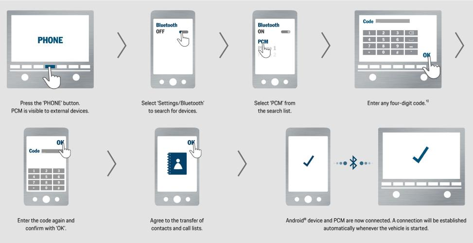
1) In Porsche models after November 2012, thanks to Secure Simple Pairing, it is simply a matter of confirming whether the same six-digit code is displayed on both devices.
