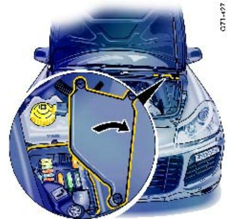
Fuse box in engine compartment
