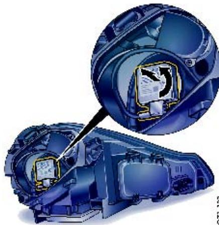
2. Turn gas discharge lamp counter-clockwise and remove.
