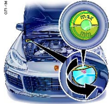
2. Open cap of the expansion tank carefully and allow any overpressure to escape. Then unscrew cap completely.
