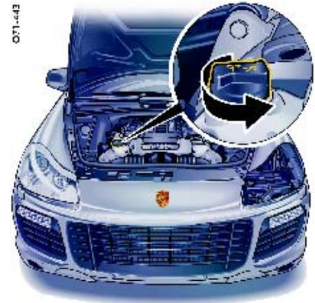
1. Unscrew cap of the oil filler opening.
