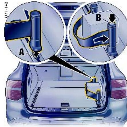
2. Insert one end element of the strap reel in the opening **A** of a mounting rail, press down and slide into position.
