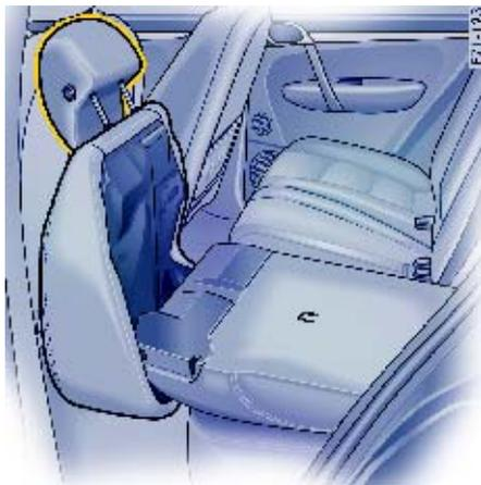
8. Insert headrest into the fixing holes in the seat cushion (arrow).
