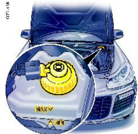
A slight decrease in the fluid level due to wear and automatic readjustment of the disc brakes is normal.
