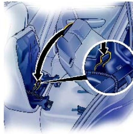
7. Insert hook on the seat cushion in the eyelet of the backrest (**arrow**).
