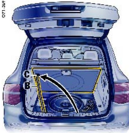
2. Unclip support arm **B** and insert it into fixing recess **C** in the loadspace floor.
