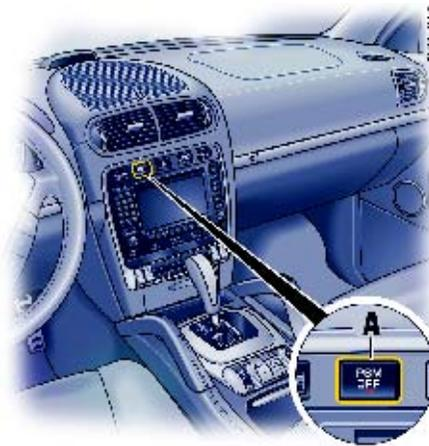
**PSM should always be switched on during “normal” driving.**
