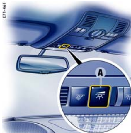
A - Button for dimming the comfort lighting
