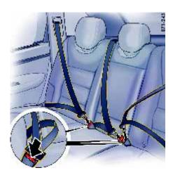
Pay attention to ensuring the correct assignment of seat belts and buckles on the rear seat bench.
