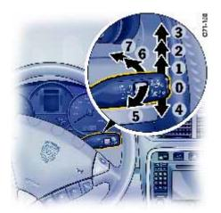
The rain sensor remains switched off if the wiper stalk is already in position **1** when the ignition is switched on.
