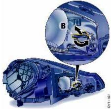
2. Turn bulb socket **B** counter-clockwise and remove.
