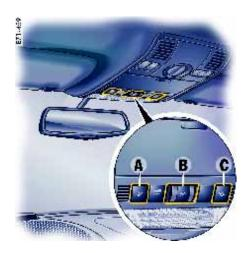
**A, C** - Switches for reading lights **B** - Switch for interior light
