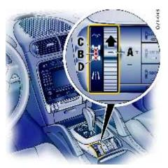
Push rocker switch A forwards in stages until engagement of the rear differential lock is indicated on the multi-purpose display of the instrument panel and by illumination of the three light-emitting diodes **B. C** and **D**. The centre and rear differential locks are changed over to fully engaged state by the automatic control system.
