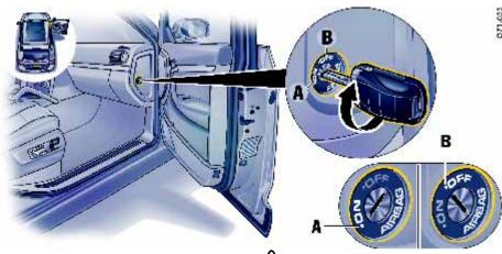
**A** - Passenger airbag switched on (ON) **B** - Passenger airbag switched off (OFF)
