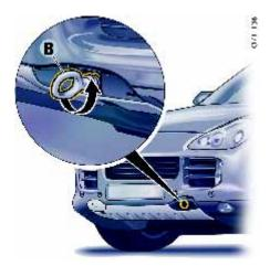
2. Screw in towing lug B as far as the stop (lefthand thread) and tighten hand-tight.
