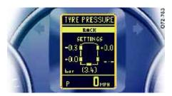
The spare wheel is not equipped with a wheel transmitter and is not monitored by Tyre Pressure Monitoring. The tyre pressure warning light lights up on the speedometer when the ENTER button is pressed. The value "\_.\_" is displayed in the submenu TYRE PRESSURE (filling information) at the position of the spare wheel.
