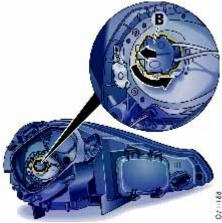
2. Turn bulb socket **B** counter-clockwise and remove.
