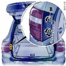
4. Unscrew the two fastening screws **B** with the socket wrench from the tool kit.
