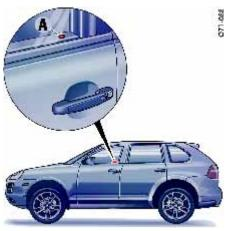
A - Light-emitting diode for alarm system example: driver's door
