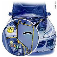
Fuse box in engine compartment
