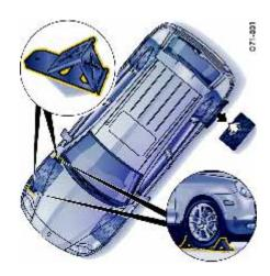
4. Place one wedge each directly in front of and behind the diagonally opposite wheel.
