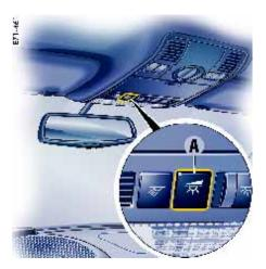
A - Button for dimming the comfort lighting
