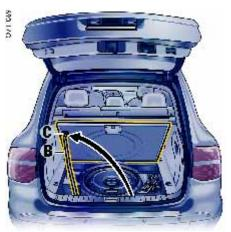
2. Unclip support arm **B** and insert it into fixing recess **C** in the loadspace floor.
