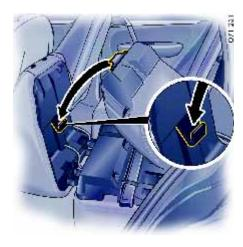
6. Insert support bracket of the backrest in the support hook on the seat cushion (arrow).
