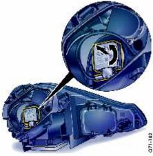
2. Turn gas discharge lamp counter-clockwise and remove.
