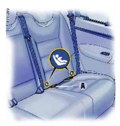
The retaining lugs **A** for the Isofix child seat anchorage can be found directly under the markings between backrest and seat cushion.
