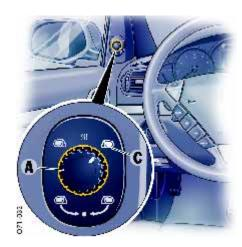
**A** - Control switch for door mirror adjustment
