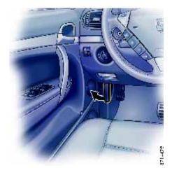
1. Pull the release lever **(arrow)**. The engine compartment lid is now unlocked.
