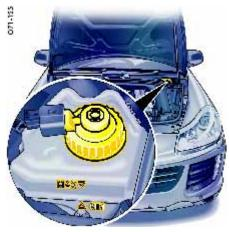
A slight decrease in the fluid level due to wear and automatic readjustment of the disc brakes is normal.
