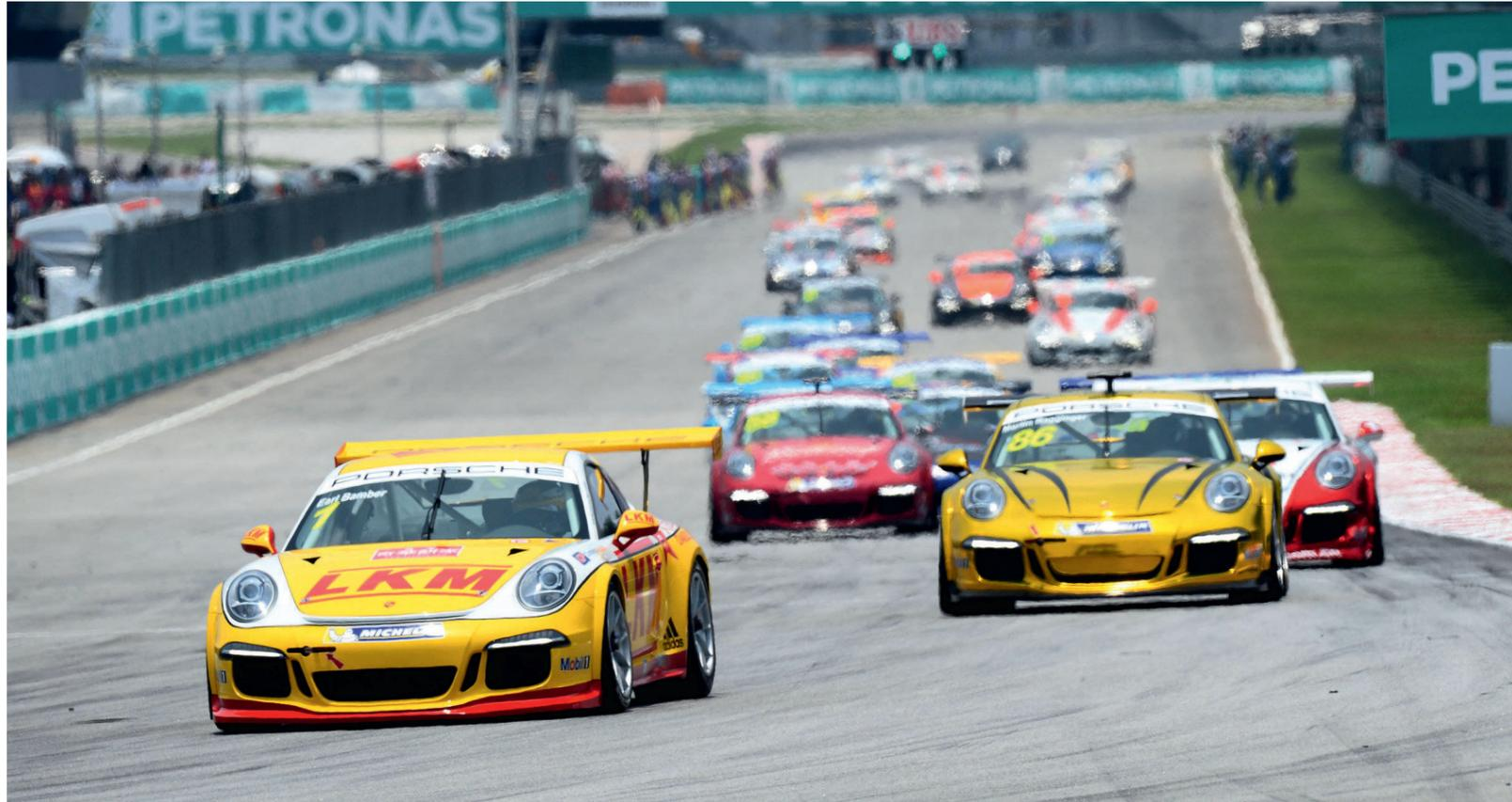
coming drivers, the championship further raises the intensity this year through the improvement of another key element – the car itself. With a more powerful 3.8-litre flat six engine, the new Porsche 911 GT3 Cup (Type 991) produces 460 horsepower, 10 more than previously, and is fitted with a six-speed sequential gearbox operated by a pneumatic paddle shift system, a first for the Porsche Carrera Cup Asia.
