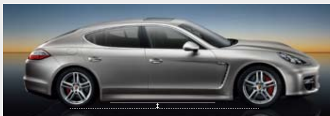
▲ Low level – 25 mm below normal level, max. ground clearance 119 mm. For sporty driving when road-holding conditions are ideal.
