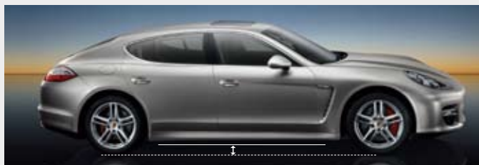
▲ Normal level – Max. ground clearance 144 mm as per DIN unladen weight. The system's default setting.
