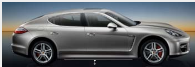
▲ High level – 20 mm above normal level. For exceptionally rough road conditions. The chassis automatically returns to normal level at speeds of over 30 km/h.
