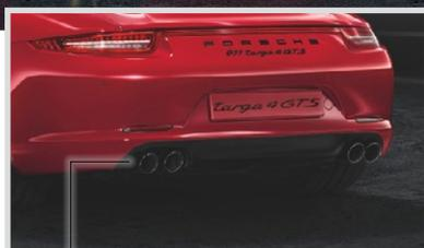
Sports exhaust system with twin tailpipes in stainless steel
