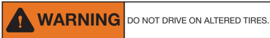
Do not make or allow to be made any alterations on your tires. Alterations may prevent proper performance, leading to tire damage that can result in an accident. Tires that become unserviceable due to alterations such as truing, whitewall inlays, addition of balancing or sealant liquids, or the use of tire dressing containing petroleum distillates, are excluded from warranty coverage.
