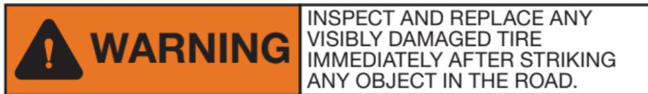
Road hazards and objects in the road, such as potholes, curbs, glass, metal, rocks, wood, and debris, can damage a tire and should be safely avoided. If your vehicle hits any such hazard or object, however, you should promptly inspect your tires. If you see any damage to any tire or wheel, replace it with a properly inflated spare at once and have your tires, including the spare, inspected by a tire professional.
