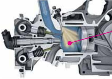
Direct gasoline injection with 140 bars (2,031 psi) injection pressure
