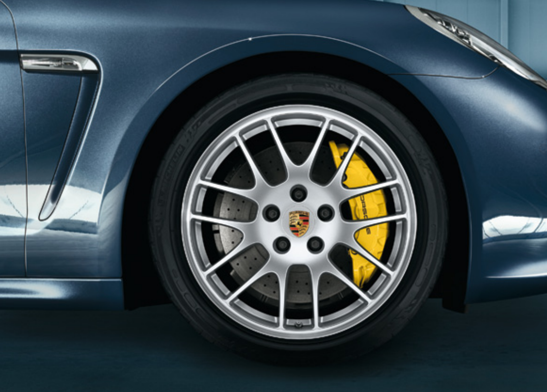
Porsche Ceramic Composite Brake (PCCB)
