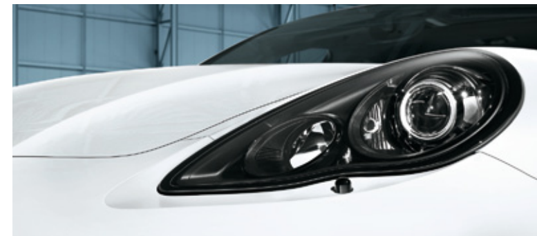
Bi-Xenon main headlights in black including PDLS
